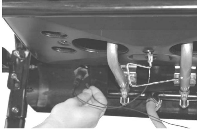
▲ Connect the side burner electrode wire to the tag on the side of the push button igniter.
