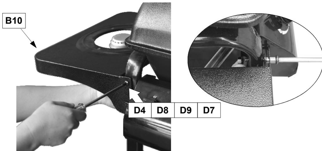
▲ Fit the side burner venturi tube over the gas valve outlet. This is a loose fit and not a gas tight seal. Then attach side burner shelf as shown in the diagram.
