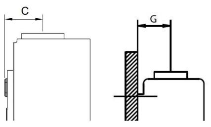
Dimension C is for the new EUP11RS water Heater which is 142mm
