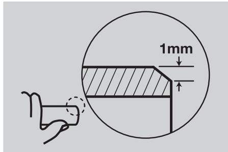
Check the tube ends are free from damage and clean, wiping away any swarf to avoid damaging the 'O' ring on tube insertion. Tube end must also be free from stickers, tape and adhesive residues.
