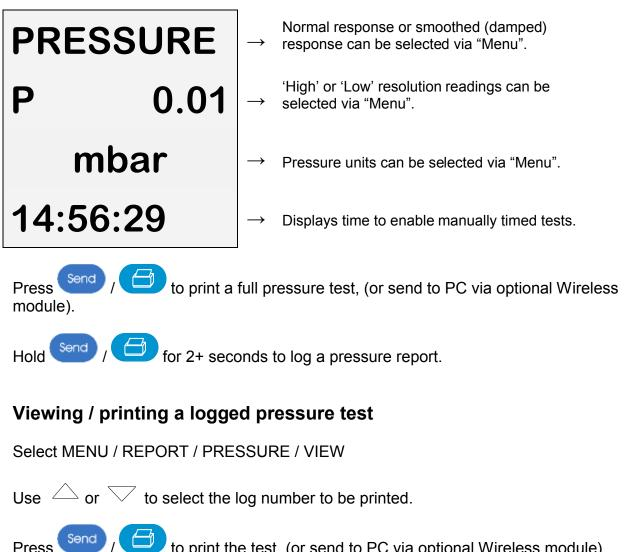
to print the test, (or send to PC via optional Wireless module).
