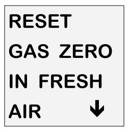
This message indicates that the analyser needs to be reset in fresh air. To do so,
