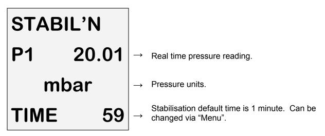
When complete press  $\checkmark$  to start the tightness test:
