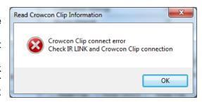
IR Link Connect Error: This error occurs when the IR Link is either not connected to the computer or the driver did not install correctly. Make sure to check the USB connection on both the computer and the IR Link itself to insure all connections are secure. If all connections are secure attempt to uninstall and reinstall the software.
